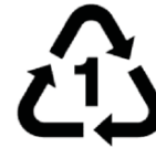
Figure 2. Recycling code for polyethylene terephthalate (PET). These codes, introduced in 1988 by the plastics trade association (the Society of the Plastics Industry, Inc.), help consumers identify and recycle different forms of plastics.
